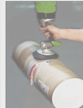
▲ 圓柱體搬運作業 Cylinder lifting
