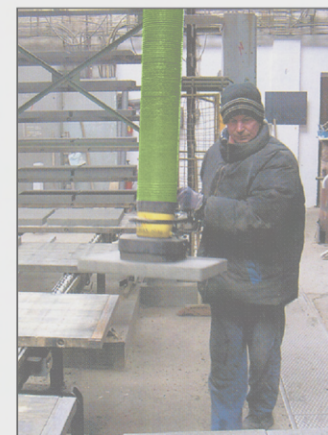
▲ 塑板搬運作業 Plastic Plank / brick
